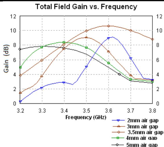
Fig.3: Simulated antenna gain versus the airgap thickness graph
